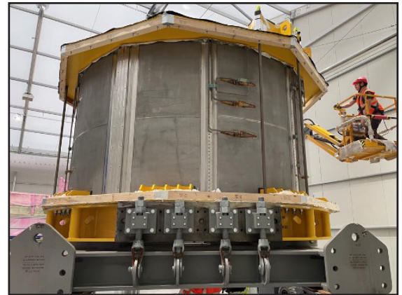
The fourth central solenoid module has been delivered and unpacked at ITER. Photo: ITER Organization
