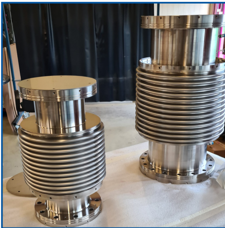
A prototyped double-walled vacuum bellows fabricated by Kompaflex for use in the cryostat vacuum system. Photo: Kompaflex
