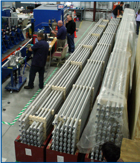
Jacketing material at the conductor integrator High Performance Magnetics. Photo: US ITER
