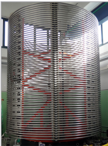
A completed spool of conductor at Criotec in Chivasso, Italy. Photo: US ITER
