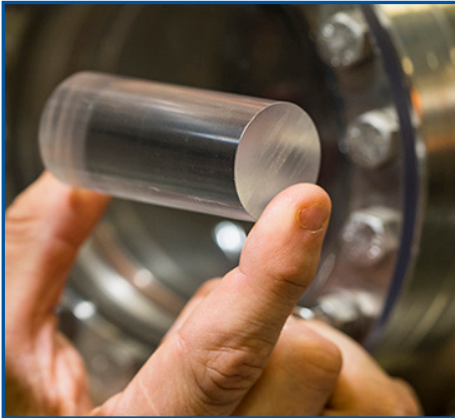
Plastic model of a pellet illustrating the size that will be used in ITER's disruption mitigation system. Photo: ORNL
